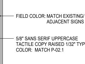
SIGN BACKING PLATE - MATCH SIZE AND SHAPE OF SIGN - MECHANICALLY ATTACH TO SUBSTRATE
