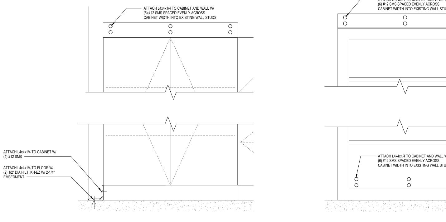
8 DETAIL - ELEVATION - INT - METAL FILE CABINET ANCHORAGE A10.50 SCALE: 1 1/2" = 1'-0"
