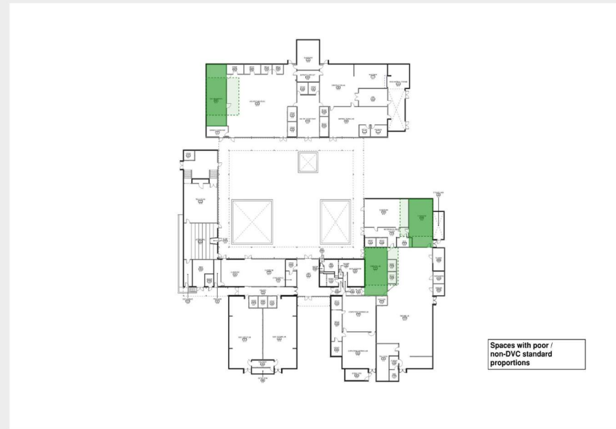
POORLY PROPORTIONED SPACES
