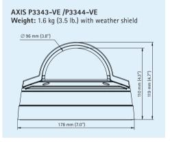
AXIS P3343/-V/P3344/-V AXIS P3343/P3344 weight: 450 g (1.0 lb.) AXIS P3343-V/P3344-V weight: 660 g (1.5 lb.)
