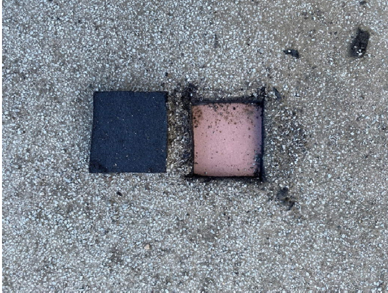
Figure 17. Roof core made at upper canopy roof.
