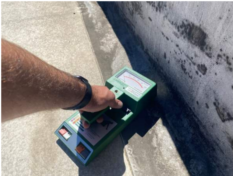
Figure 20. Tramex moisture meter used across the roof deck to assess moisture content of roof assembly.
